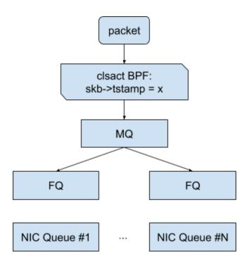
HTB qdisc was replaced with a set of FQ qdiscs (one per NIC queue) which provides per-flow fairness and enforcement of skb departure timestamp. This eliminated contention on the global HTB lock and the global qdisc lock now is split into per-flow-aggregate state. Our BPF program was extended with a per-flow-aggregate map and a small amount of BPF was written to keep track of the per-low-aggregate state.
