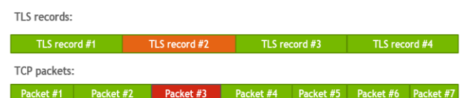
Figure 2- packet 3 received decrypted will all other is plaintext, SW will finish the job.
