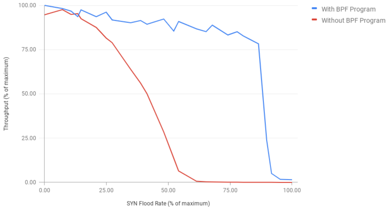
Figure 2: 100-flow throughput at different SYN flood rates compared between kernel and XDP SYN cookie generation
