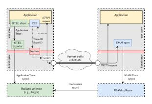
Figure 2: Cross-Layer Telemetry architecture.
