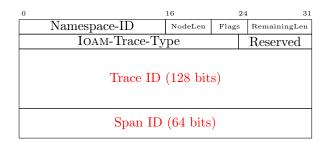
Figure 4: Enhanced IOAM PTO Header.
