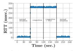
Figure 11: RTT measurement, 200 requests/second, four steps with congestion.
