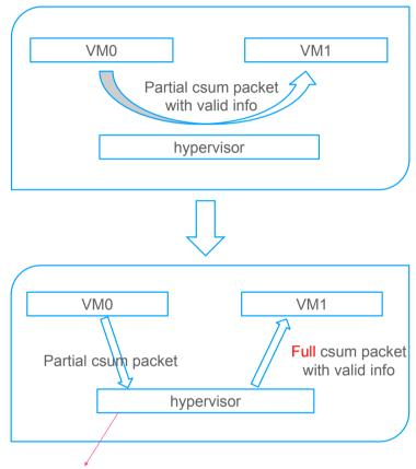
More devices have FPGA, calculating the csum does not occupy too much resource. The virtio-net can work more like the physical net card.
