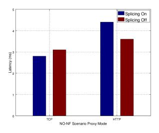
Figure 6: Latency Impact of TCP Splicing
