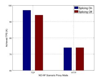
Figure 5: TPS Impact of TCP Splicing
