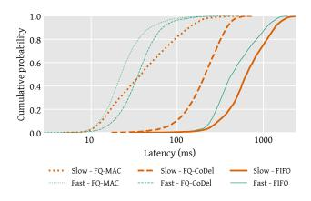
Figure 2: Latency (ICMP ping) with simultaneous TCP download traffic.
