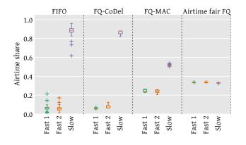
Figure 3: Airtime usage for each of the three stations in the different scenarios (UDP traffic).
