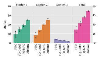
Figure 4: Throughput for TCP download traffic (to clients).
