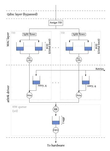
Figure 1: Our 802.11-specific queueing structure, as it looks when applied to the Linux WiFi stack.
